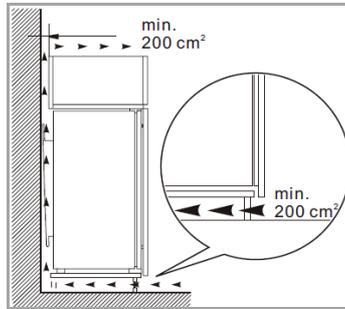
For ventilation, an exhaust duct of approx. 38 mm depth must be provided on the appliance back.
